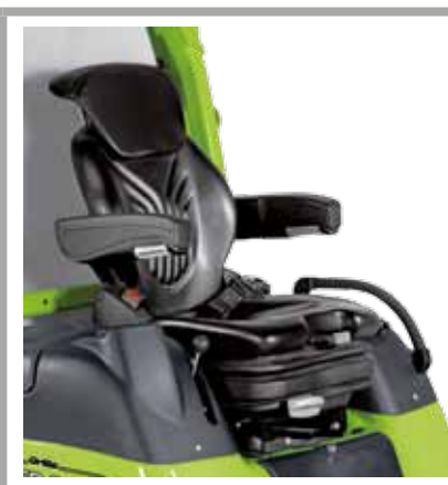
Pneumatic suspension seat as standard feature
