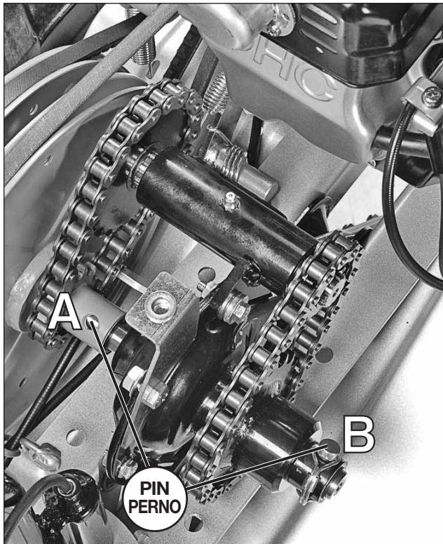
**GB: Speed change pin.** Position B: gear used if the machine has to operate with the rotary tiller on a hard soil. Position A: gear used if the machine has to operate with the rotary tiller on loose soil.
