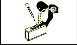
Sulfuric acid in battery electrolyte is poisonous. It is strong enough to burn skin, eat holes in clothing and cause blindness if it gets in contact with the eyes.
