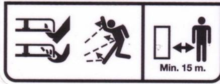
**WARNING! SHARP PARTS.** Keep hands and feet away. Do not operate the mower over gravel or foreign bodies which may be sucked up and ejected by the blades, generating a danger. Keep people at a min. distance of 15 metres. Remove the key and read the instruction manual before attempting to carry out any maintenance or repairs to the machine.
