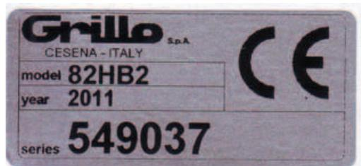
The vehicle's serial number is punched on the nameplate on the gearbox nameplate. Always state the serial number when ordering spare parts.
