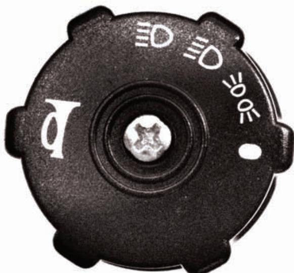
**LIGHT AND HORN SWITCH · COMMUTATORE LUCI ED AVVISATORE ACUSTICO
