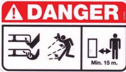
**WARNING! SHARP PARTS.** Keep hands and feet away. Do not operate the mower over gravel or foreign bodies which may be sucked up and ejected by the blades, generating a danger. Keep people at a min. distance of 15 metres. Remove the key and read the instruction manual before attempting to carry out any maintenance or repairs to the machine.
