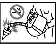
Handle fuel with care, it is highly flammable: Do not refuel machine while smoking, when machine is near an open flame or sparks, or when the engine is running. Stop the engine.
