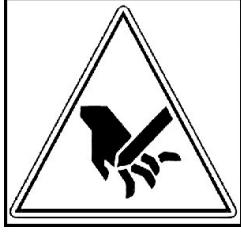
**WARNING!** SHARP PARTS. Keep hands and feet away. Do not operate the mower over gravel or foreign bodies which may be sucked up and ejected by the blades, generating a danger. Keep people away. Remove the key and read the instruction manual before attempting to carry out any maintenance or repairs to the machine.
