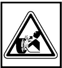
A burst which separates the tyre from the rim parts can cause serious injury or death.
