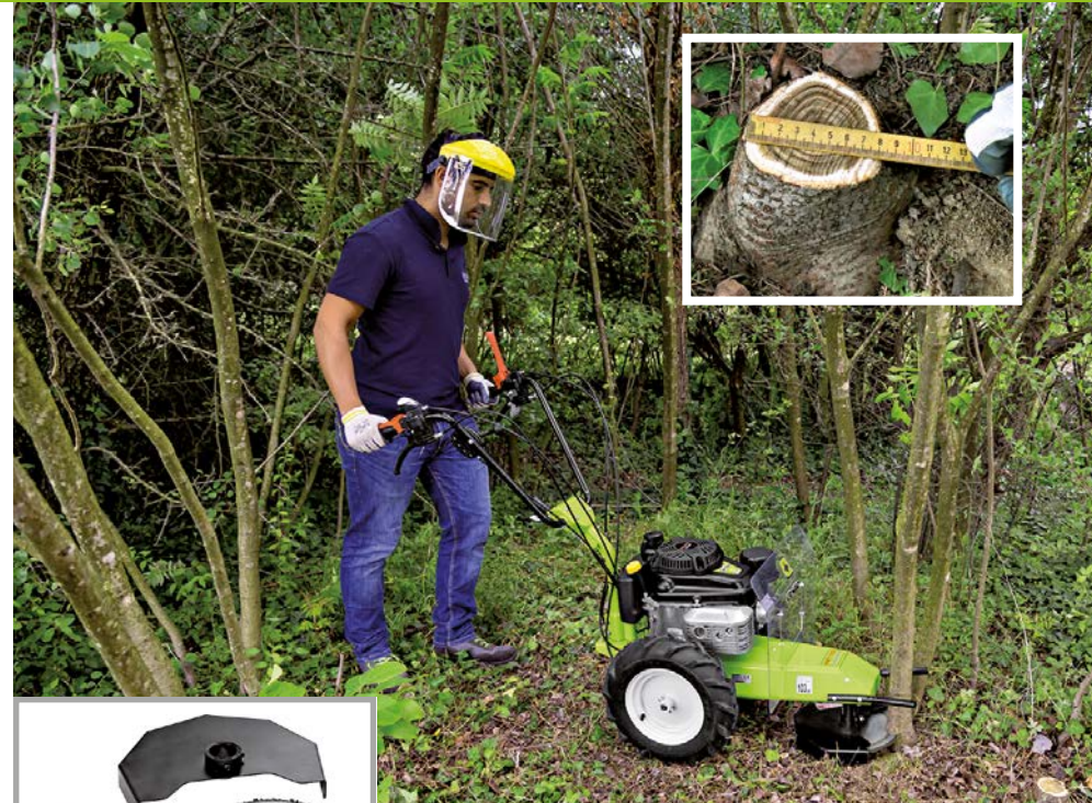
The saw blade, supplied as optional accessory, allows you to cut small trees up to 8 cm in diameter.
